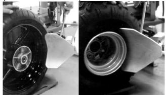
Turn wheel around and repeat loosening procedure on the other side of the wheel. This should be the long side of the drop center.
